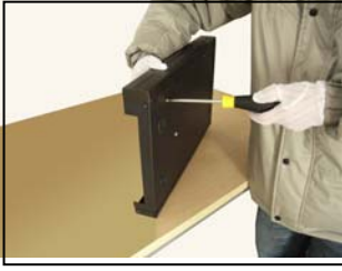
④fix the screw of hard disk
