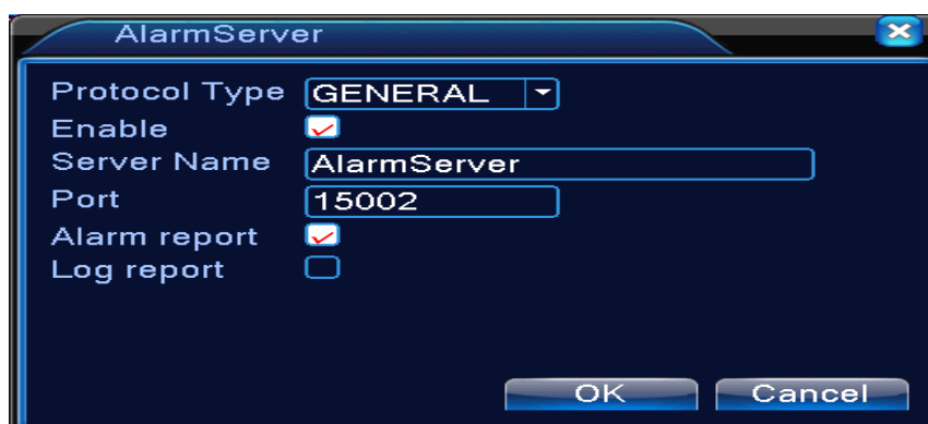
Picture 4.23 alarm server setting
