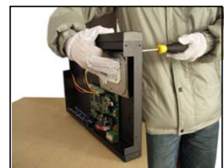
③ fix the screw of hard disk
